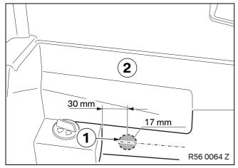
Drill through the hole (1) in the glove compartment (2) using a 17 mm step drill bit using the dimensions shown.
