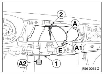
Pull branch **A1** of connection cable **A** to the inside until iPod connection plug **A2** is located just above the outside edge (1) of the glove compartment.
