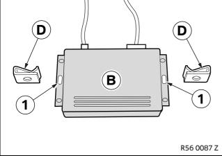
Push speed nuts **D** onto the slots (1) in the interface **B**.
