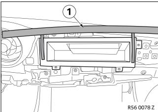
The flap (1) must be fixed after mounting the interface in order to avoid it being opened by the customer. ◀
