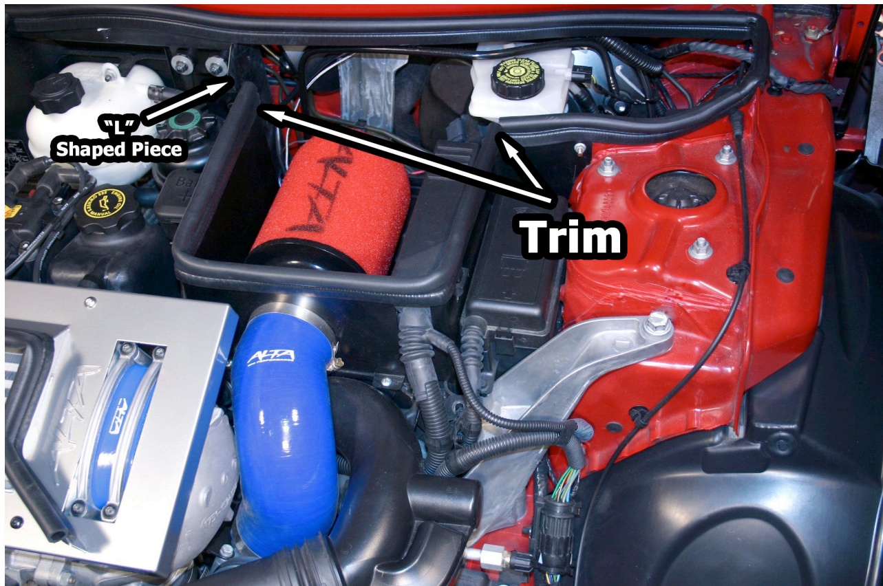
Completed Install: Note trim around box and wall removed
