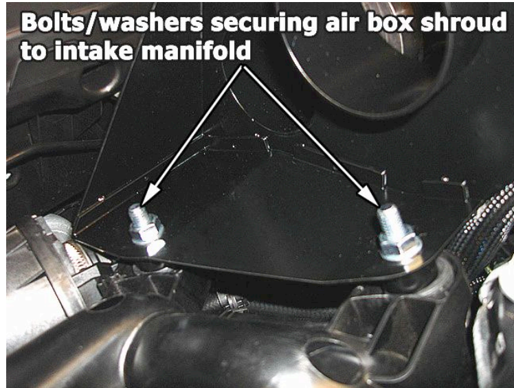
AIR BOX SHROUD BOLTED TO TOP OF INTAKE MANIFOLD USING SUPPLIED BOLTS
