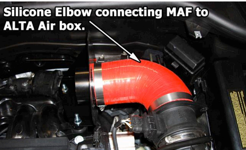
MAF SENSOR AND SILICONE ELBOW INSTALLED TO AIR BOX SHROUD
