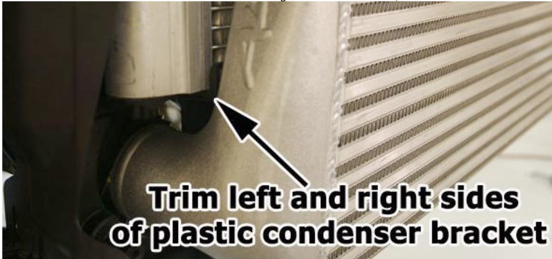
17. Install ALTA intercooler in place of OEM intercooler, and connect boost tubes to intercooler. Before tightening clamps, ensure they are positioned properly to allow access to nut.
