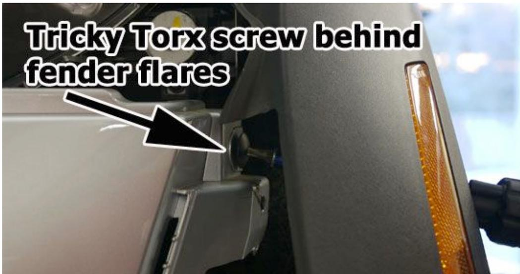
10. Under bottom of bumper, locate and remove (2) Torx screws and (4) Pop-it fasteners.
