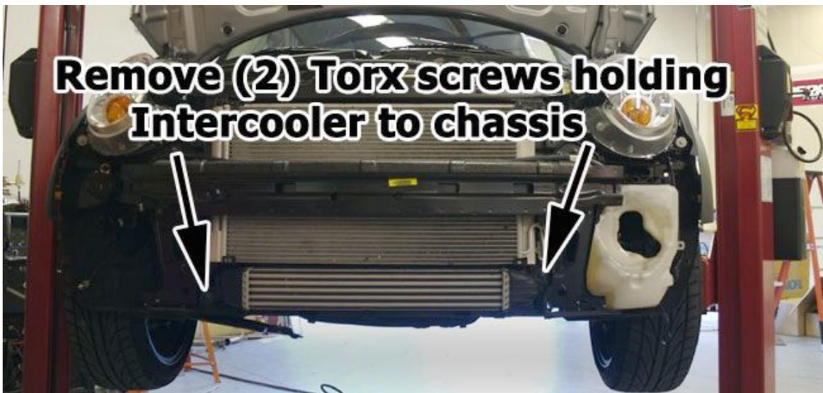
13. Take note as to direction hose clamps were facing before loosening. Loosen clamps securing boost tubes to intercooler. Note: Using a bent awl will help to free up rubber boost tube around intercooler.
