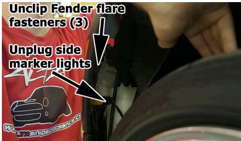
7. Pull back fender liner, locate and remove side marker plug, and pop-it connector holding upper and lower bumper together.
