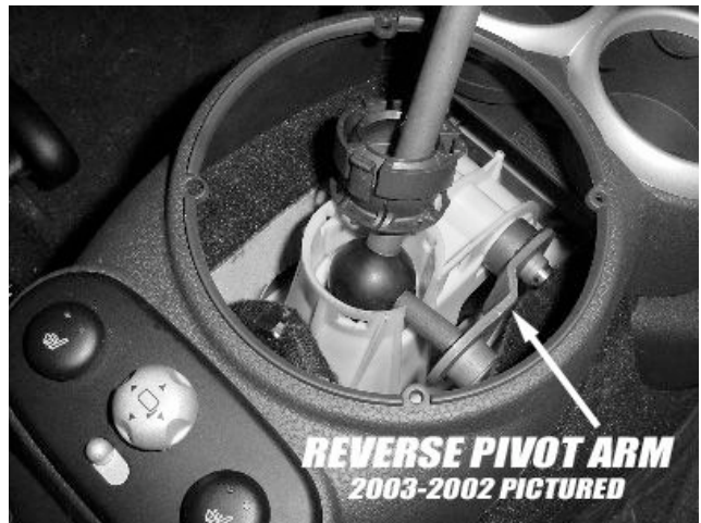
2002-2003 shown, 2004+ has black plastic body, and pivot arm.
